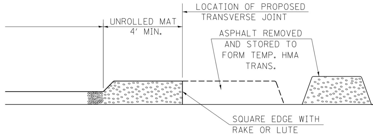
MOVE THE PAVER OUT OF THE WAY AND REMOVE THE ASPHALT FROM THE AREA OF THE PROPOSED TEMPORARY HOT-MIX ASPHALT TRANSITION.
