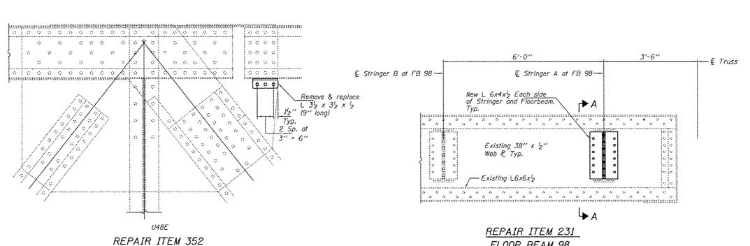
O- Use holes in existing member as template • - Use holes in new member as template
