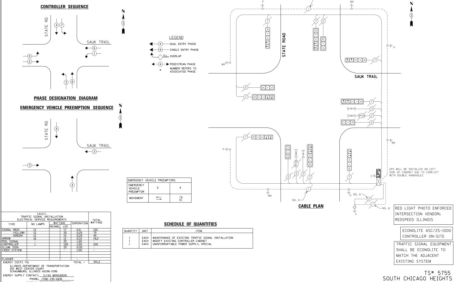
COMPANY: COMMONWEALTH EDISON DESIGNED - V.O. REVISED SCHEDULE OF QUANTITIES, CABLE PLAN, PHASE DESIGNATION DIAGRAM, AND SECTION COUNTY **STATE OF ILLINOIS** :\13155\60Y42\DGN\CADD Sheets\D160Y42 nt-ts-50\_5755.dan DRAWN E.C. REVISED **EMERGENCY VEHICLE PREEMPTION SEQUENCE** COOK 65 65 2014-044TS SAUK TRAIL AT STATE ROAD CHECKED - I.Y. REVISED **DEPARTMENT OF TRANSPORTATION** CONTRACT NO. 60Y42 SCALE: NTS SHEET NO. 1 OF 1 SHEETS STA. N/A DATE REVISED PLOT DATE = 7/9/2014 7/11/2014
