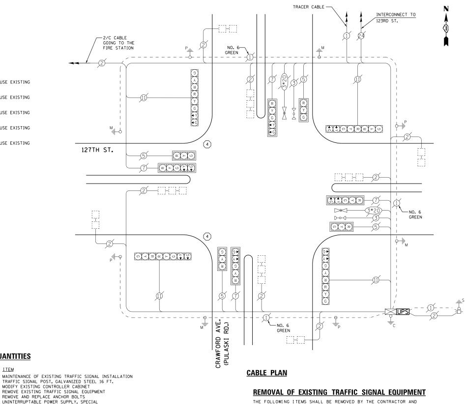
THE FOLLOWING ITEMS SHALL BE REMOVED BY THE CONTRACTOR AND SHALL BE DISPOSED OF BY THEM OUTSIDE THE RIGHT-OF-WAY AT THEIR EXPENSE. THE SALVAGE VALUE OF THE REMOVED EQUIPMENT SHALL BE REFLECTED IN THE CONTRACT BID PRICE. 2 EACH SIGNAL POST
