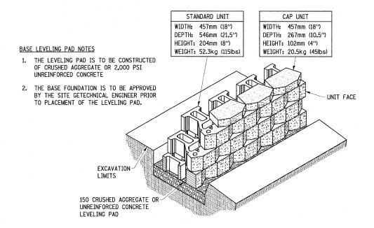
STANDARD UNIT/BASE PAD ISOMETRIC SECTION VIEW
