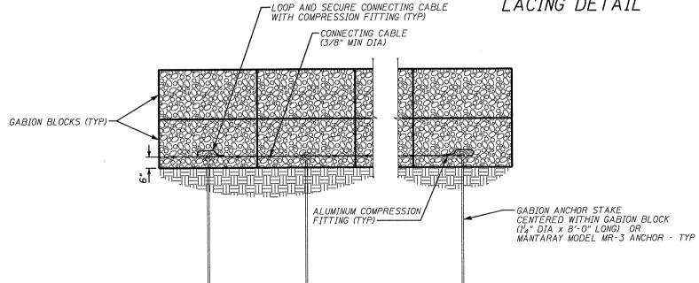
GARION ANCHOR STAKE SECURING DETAIL
