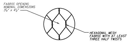
1. GABION BASKETS SHALL BE CONSTRUCTED OF A GALVANIZED. ALUMINIZED, OR PVC-COATED GALVANIZED OR ALUMINIZED STEEL WIRE.
