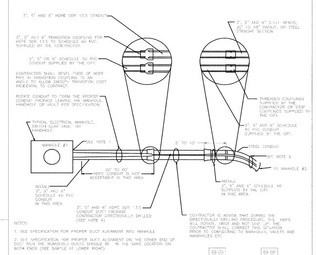
3. COST TO PROPERLY INSTALL CONDUIT FROM ONE ELECTRICAL FACILITY TO ANOTHER IS INCIDENTAL TO THE COST OF THE WORK.
