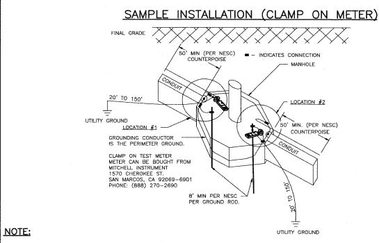
OBSERVE ALL SAFETY REQUIREMENTS AND THEN REMOVE COVERING ON THE GROUND CONDUCTOR IF PRESENT AND PROVIDE SUFFICIENT ROOM FOR THE MODEL 3710/3730 JAWS, WHICH MUST BE ABLE TO CLOSE EASILY AROUND THE CONDUCTOR. THE JAWS CAN BE PLACED AROUND THE GROUND ROD ITSELF. NOTE: THE CLAMP MUST BE PLACED SO THAT THE JAWS ARE IN AN ELECTRICAL PATH FROM THE SYSTEM NEUTRAL OR GROUND WIRE TO THE GROUND ROD, OR COUNTERPOISE.
