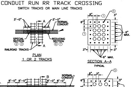
THIS STANDARD SHALL BE USED FOR THE FORMATION OF CONDUIT RUNS THAT CROSS UNDER RAILROAD TRACKS
