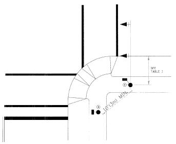
RECOMMENDED PUSHBUTTON LOCATIONS FOR ACCESSIBLE PEDESTRIAN SIGNALS SHALL BE IN ACCORDANCE WITH THE CURRENT MUTCD (SEE NOTE 1). TO MEET MUTCO REQUIREMENTS, PEDESTRIAN SIGNAL PUSHBUTTONS MAY HAVE TO BE MOUNTED ON A SEPARATE POST.
