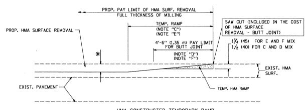
HMA CONSTRUCTED TEMPORARY RAMP
