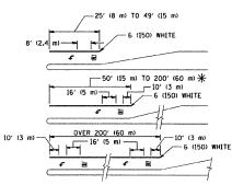
\* TURN LANES IN EXCESS OF 400' (120 m) IN LENGTH MAY HAVE AN ADDITIONAL SET OF ARROW - "ONLY" INSTALLED MIDWAY BETWEEN THE OTHER TWO SETS OF ARROW - "ONLY".
