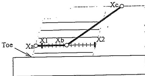
Results in the table below represent critical two-part wedges identified between specified starting (X1) and ending (X2) search points. Wedges along all reinforcement layers and at elevation zero are reported. The critical two-part wedge, one for each predetermined elevation, is defined by Xa, Xb and Xc where Xa is the front end of the passive wedge (slope face), Xb is where the passive wedge ends and the active one starts, and Xc is the X-ordinate at which the active wedge starts.
