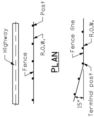
When fence line has a change in direction of 15° or more, a terminal post shall be placed as shown above.
