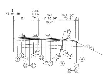
RAMP TERMINAL TYPICAL SECTION (IL 159 INTERCHANGE)
