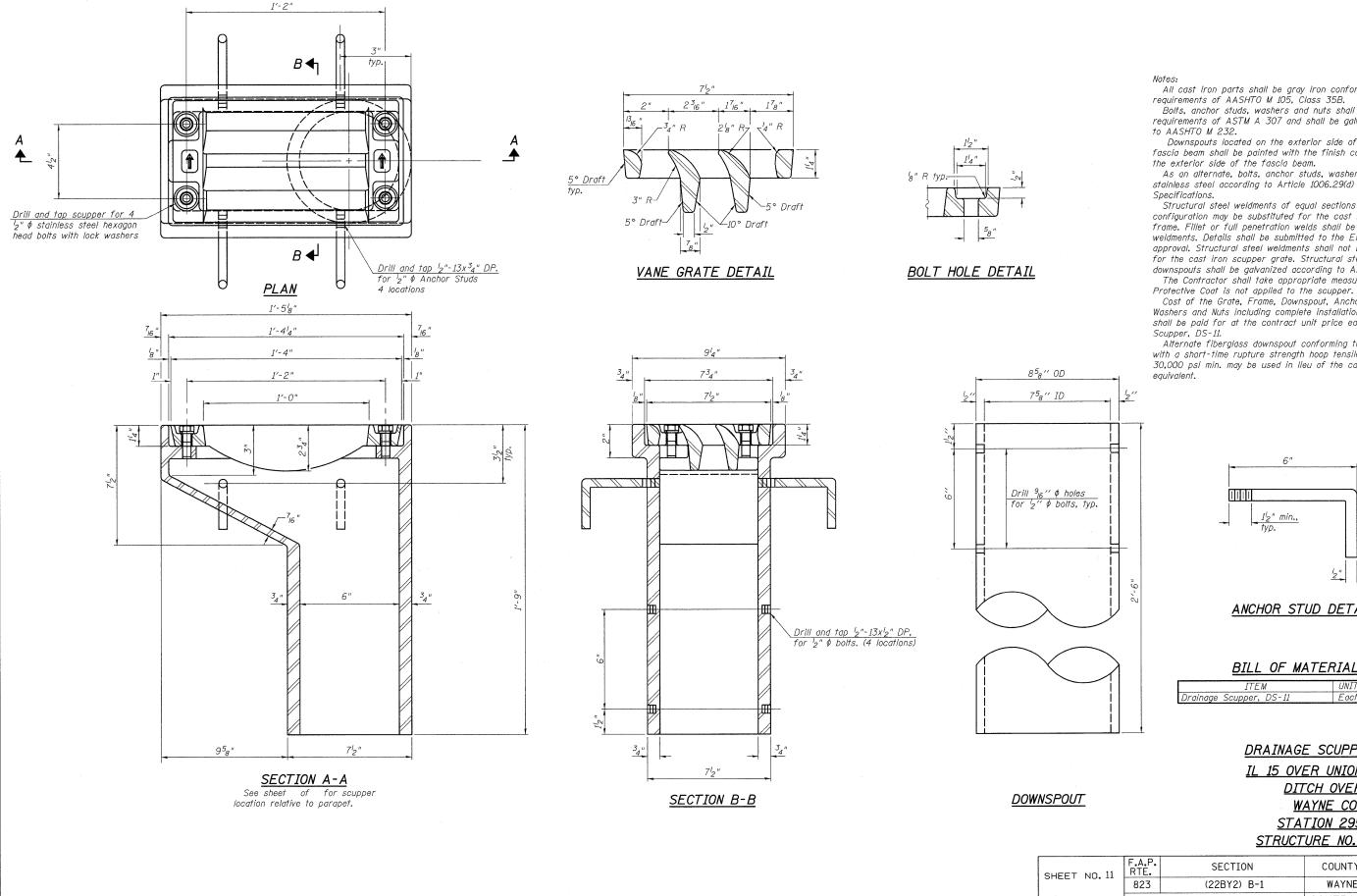
All cast iron parts shall be gray iron conforming to the requirements of AASHTO M 105, Class 35B.
