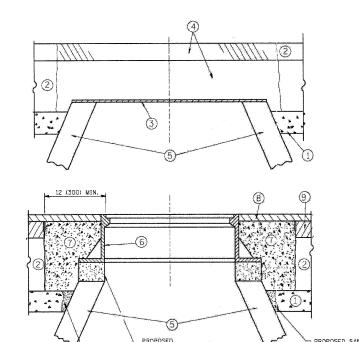
BRICK, MORTAR, OR CONC. ADJUSTING RINGS
