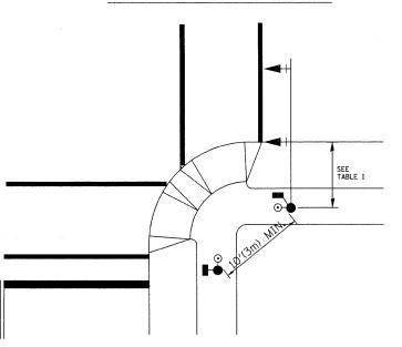
RECOMMENDED PUSHBUTTON LOCATIONS FOR ACCESSIBLE PEDESTRIAN SIGNALS SHALL BE IN ACCORDANCE WITH THE CURRENT MUTCD (SEE NOTE 1). TO MEET MUTCD REQUIREMENTS, PEDESTRIAN SIGNAL PUSHBUTTONS MAY HAVE TO BE MOUNTED ON A SEPARATE POST.
