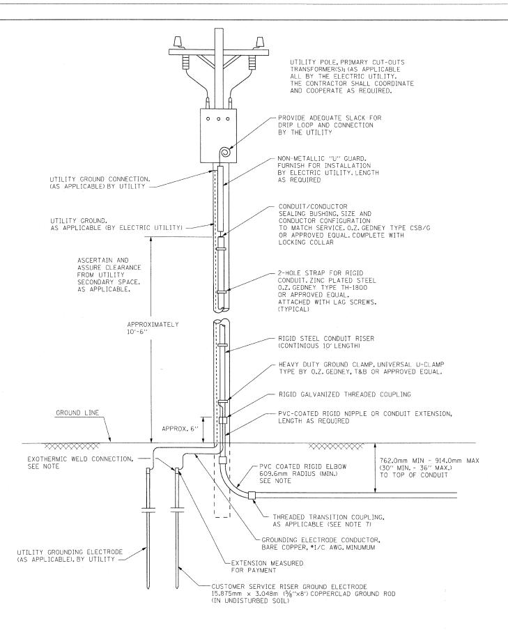
PROPOSED SERVICE INSTALLATION POLE TOP MOUNTED TRANSFORMER
