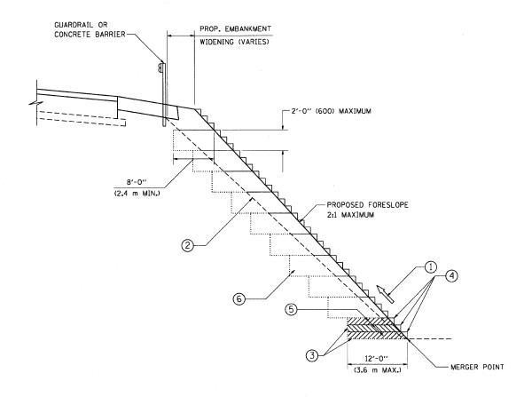
TYPICAL BENCHING DETAIL FOR EMBANKMENT
