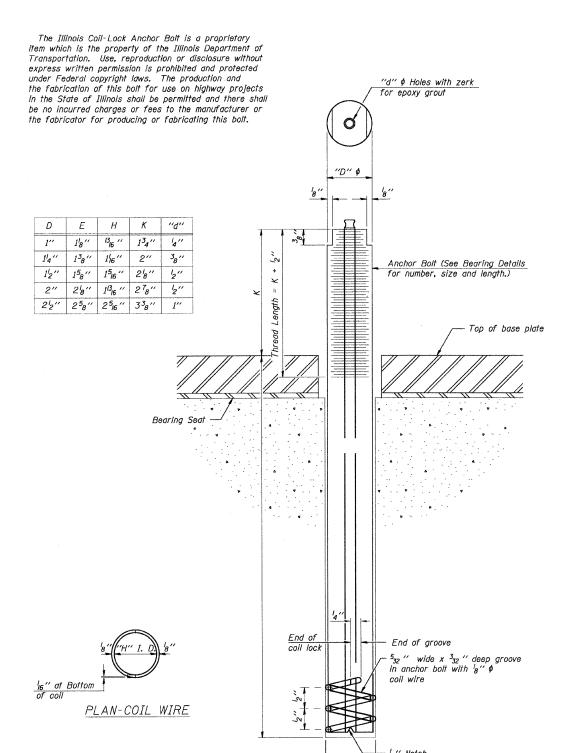
"Ε" φ ILLINOIS COIL-LOCK ANCHOR BOLT
