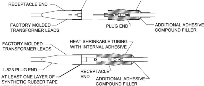
WRAP WITH AT LEAST ONE LAYER OF RUBBER OR SYNTHETIC RUBBER TAPE AND ONE LAYER OF PLASTIC TAPE, ONE-HALF LAPPED, EXTENDING AT LEAST 1-1/2 INCHES ON EACH SIDE OF JOINT.
