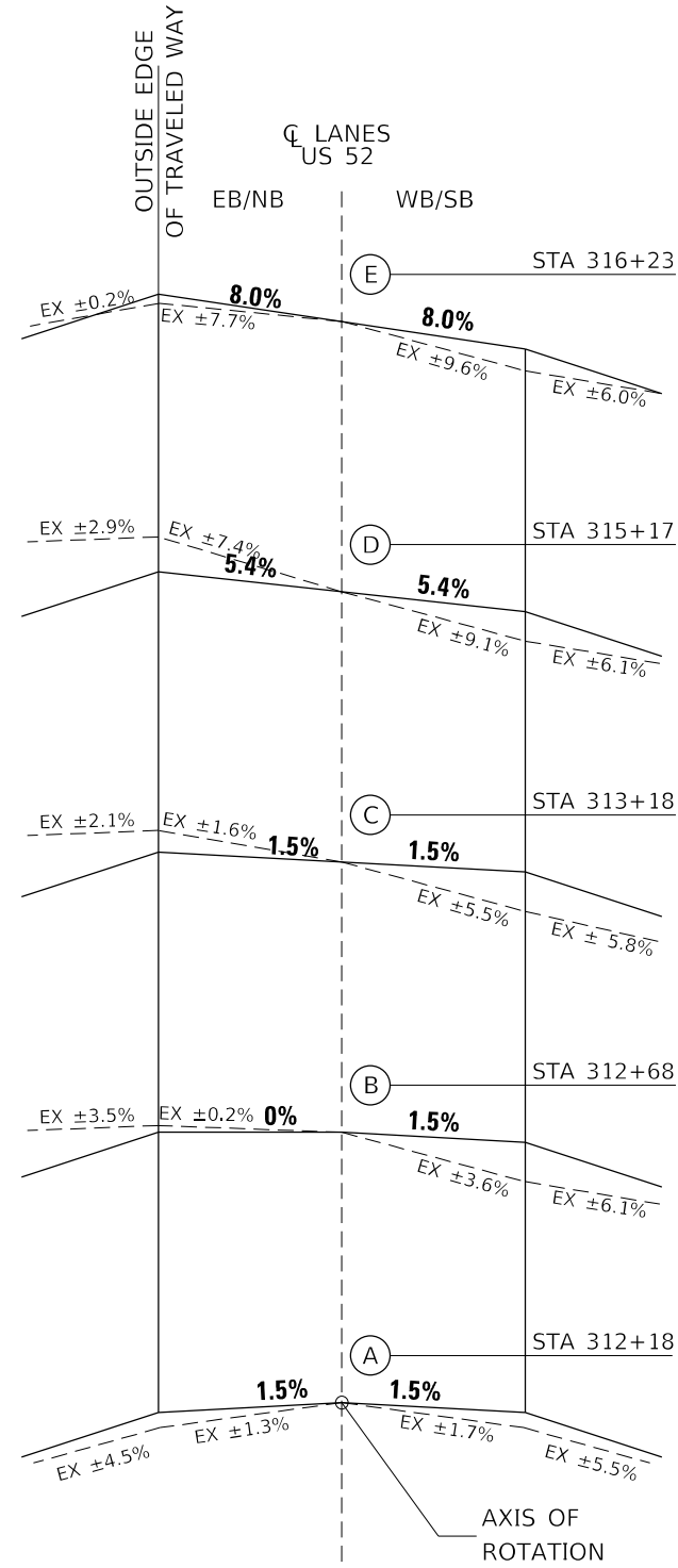
CROSS SECTIONS SUPERELEVATION DEVELOPMENT APPROACHING CURVE
