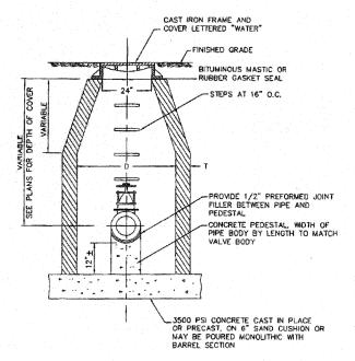
NOTE: VALVE VAULT DIA. SHALL BE 48" FOR 8" AND SMALLER VALVES AND 60" FOR 10" AND LARGER VALVES. D = DIAMETER OF MANHOLE
