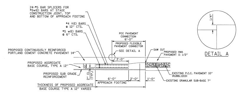
PCC PAVEMENT CONNECTION JOINT DETAIL
