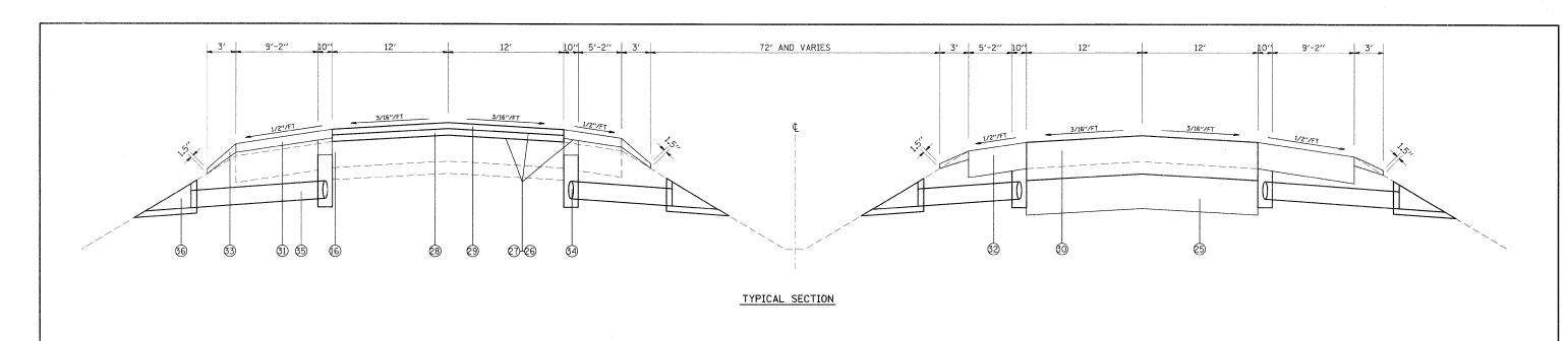
STA 362+05 TO STA 365+09 SEE PLAN VIEW AND DETAILS FOR LIMITS OF SHOULDER REPLACEMENT
