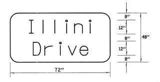
TO BE INSTALLED ON SOUTHBOUND MAST ARM (STA 67+91 67' T+.)
