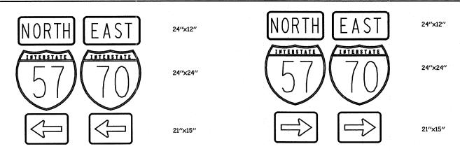
TO BE INSTALLED ON EASTBOUND MAST ARM (STA 53+71 56' Rt.)
