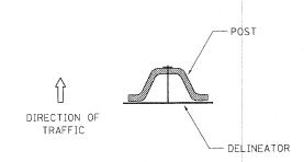
DELINEATORS SHALL BE INSTALLED ACCORDING TO STANDARD 635001 EXCEPT THAT THE POST SHALL BE ROTATED 180°. THE POST WILL HAVE THE WIDE SIDE FACING TRAFFIC AND THE DELINEATOR ATTACHECD AS SHOWN ABOVE.
