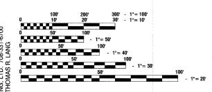
FULL SIZE PLANS HAVE BEEN PREPARED USING STANDARD ENGINEERING SCALES, REDUCED SIZED PLANS WILL NOT CONFORM TO STANDARD SCALES, IN MAKING MEASUREMENTS ON REDUCED PLANS, THE ABOVE SCALES MAY BE USED.
