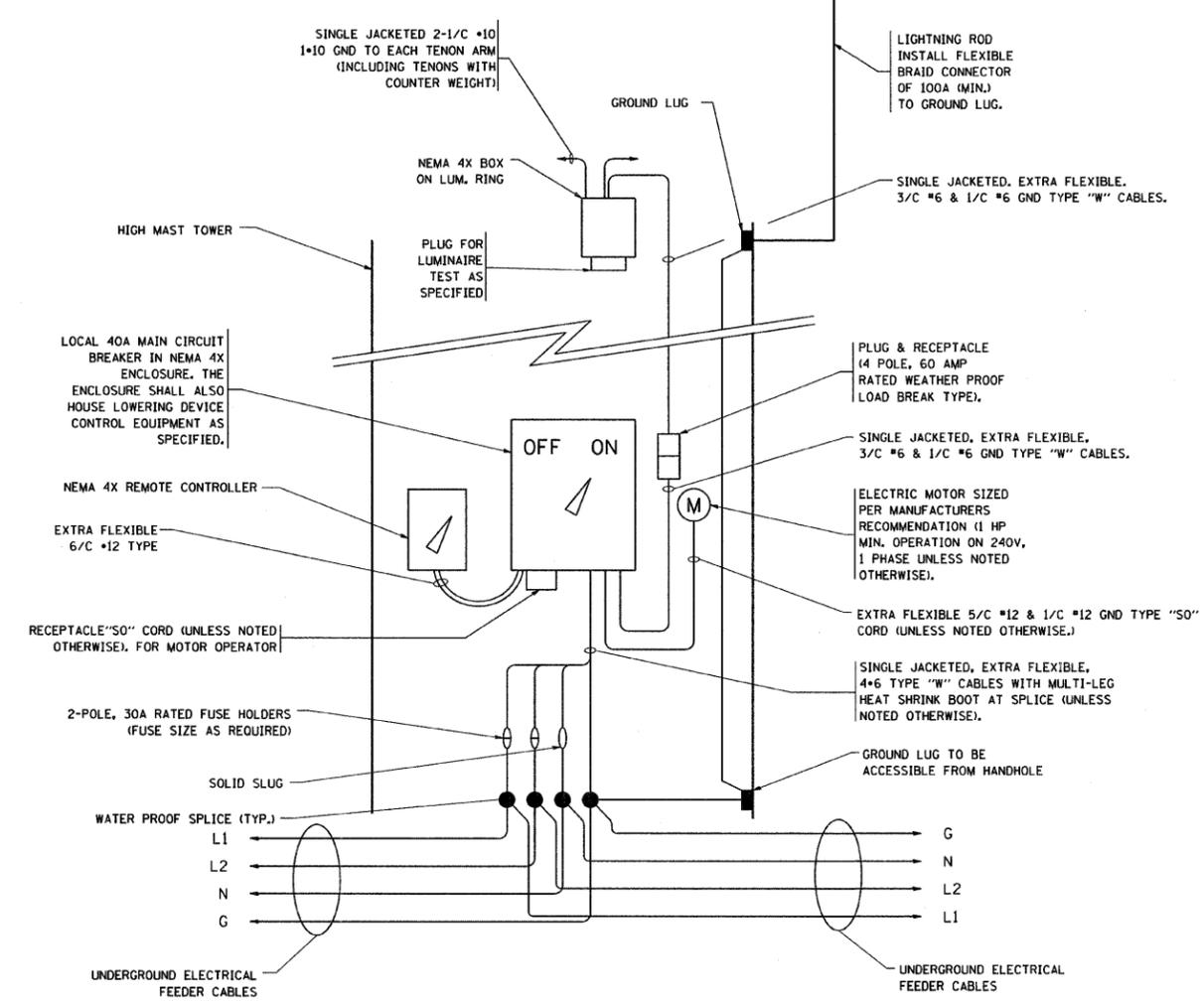
HIGH MAST POLE WIRING DIAGRAM
