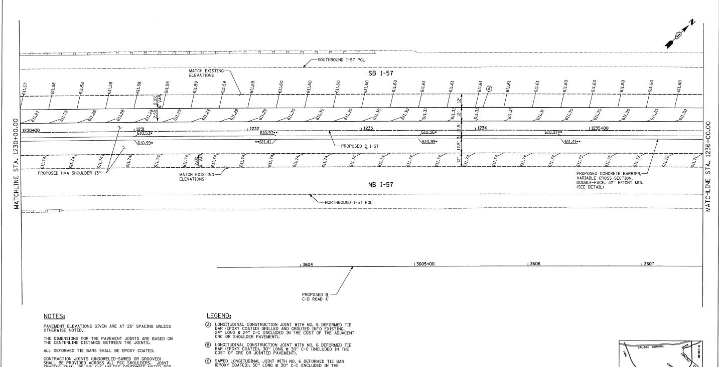
CONTRACTION JOINTS (UNDOWELED-SAWED OR GROOVED) SHALL BE PROVIDED ACROSS ALL PCC SHOULDERS, JOINT SPACING SHALL BE 20' C-C UNLESS OTHERWISE NOTED PER STANDARD 483001.
