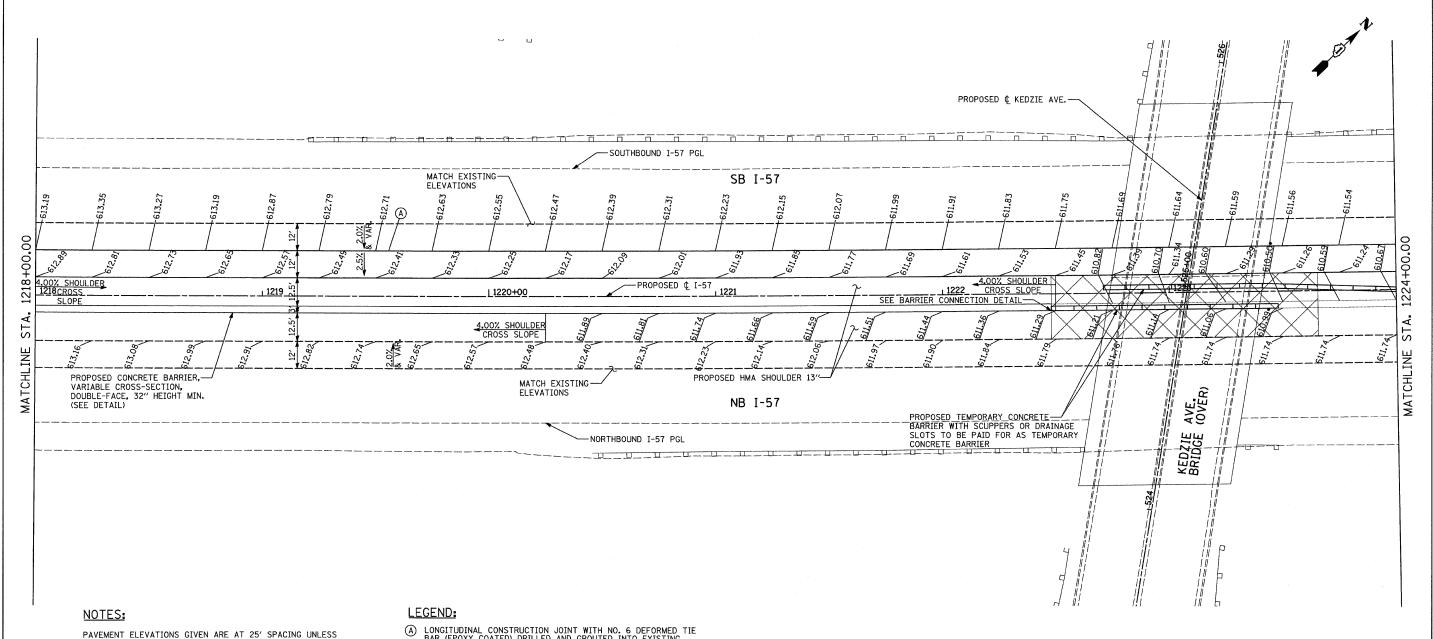
PAVEMENT ELEVATIONS GIVEN ARE AT  $25^\prime$  SPACING UNLESS OTHERWISE NOTED.
