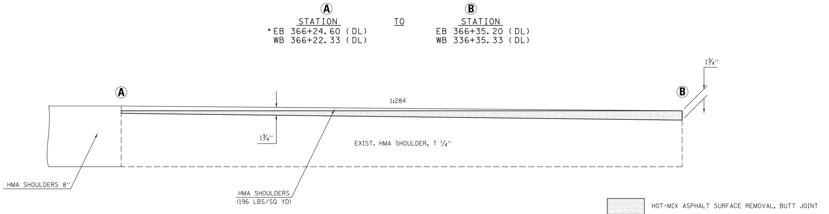
\* - EXISTING PAVEMENT AT THIS LOCATION CONSISTS OF A TYPE B GUTTER BELOW THE 7 1/4" HMA SHOULDER
