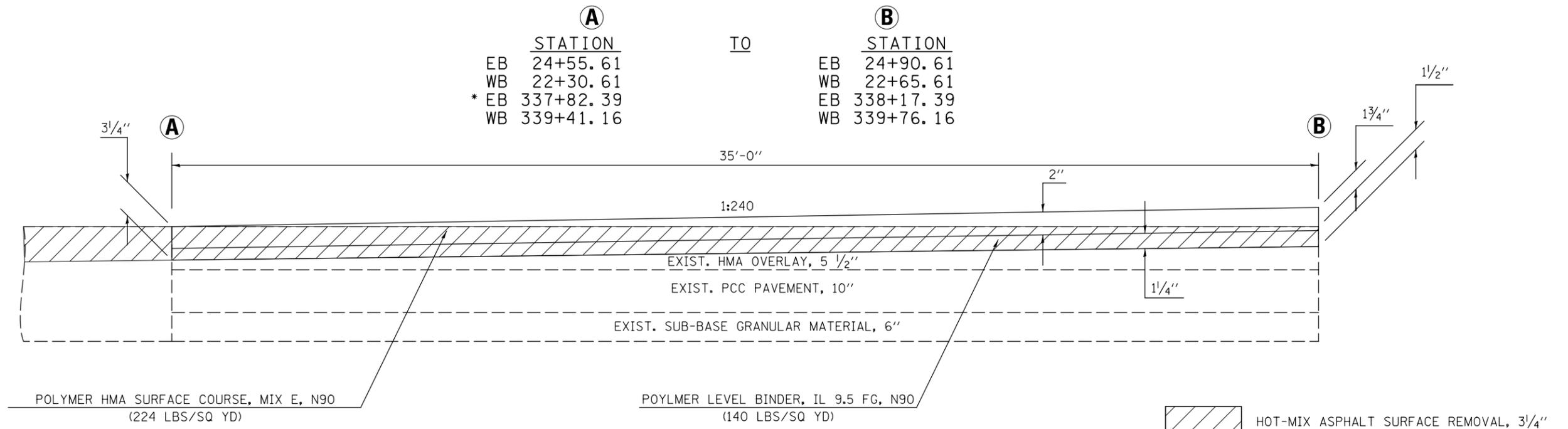
\* - EXISTING PAVEMENT AT THIS LOCATION CONSISTS OF A 7 1/4" HMA OVERLAY WITH A 9-6-9 PCC PAVEMENT
