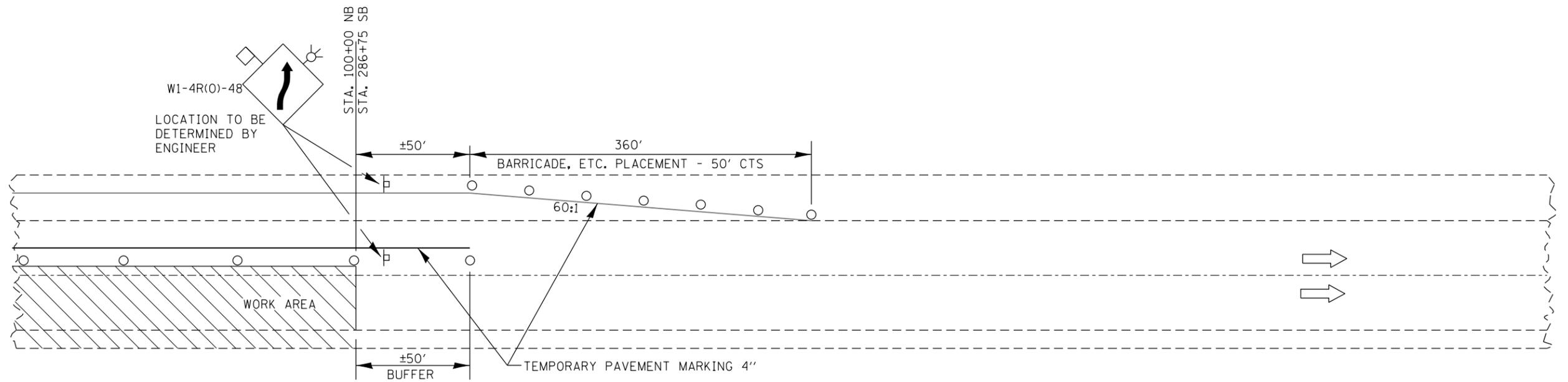
**LANE CLOSURE DETAIL STAGE 1 - ENDING TAPER (TYPICAL)**
