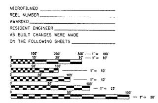
FULL SIZE PLANS HAVE BEEN PREPARED USING STANDARD ENGINEERING SCALES. REDUCED SIZED PLANS WILL NOT CONFORM TO STANDARD SCALES. IN MAKING MEASUREMENTS ON REDUCED PLANS, THE ABOVE SCALES MAY BE USED.
