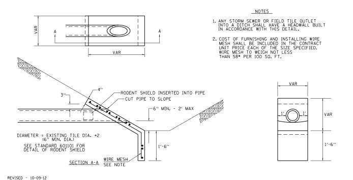
CAST-IN-PLACE REINFORCED CONCRETE END SECTIONS
