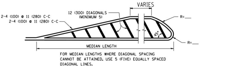
DIAGONAL LINE SPACING: 50' (15 m) C-C (LESS THAN 30MPH (50 km/h))
