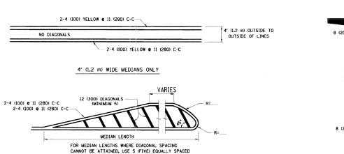
DIAGONAL LINE SPACING: 5C' (15 m) C-C (LESS THAN 30MPH (50 km/h)) 75' (25 m) C-C 30MPH (50 km/h) TO 45MPH (70 km/h)) 150' (45 m) C-C (MORE THAN 45MPH (70 km/h))
