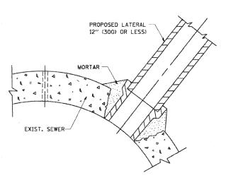
DETAIL "C" PROPOSED LATERAL CONNECTION TO EXISTING SEWER OF 30" (750) OR LARGER
