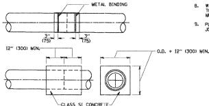
DETAIL "B" CLASS SI CONCRETE COLLAR
