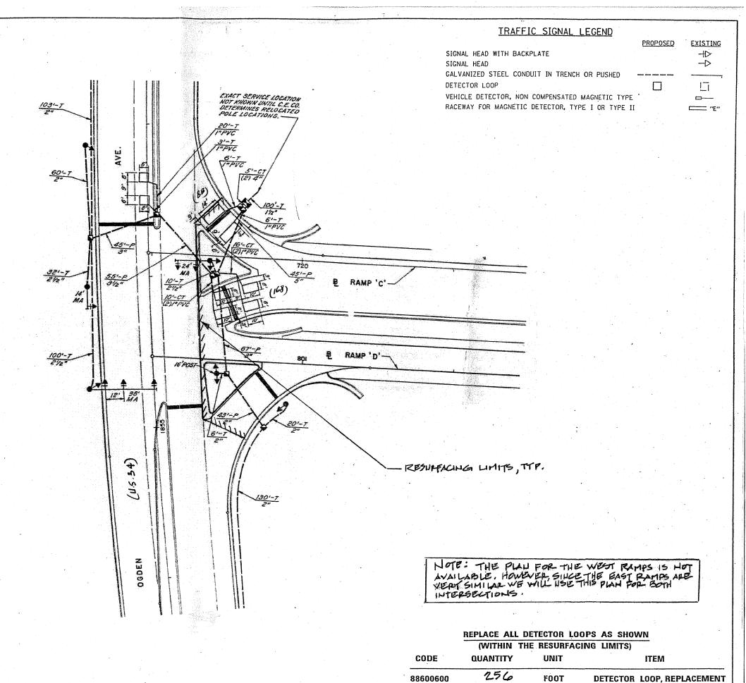
THIS PLAN IS FOR THE SOLE PURPOSE OF DETECTOR LOOP REPLACEMENTS ONLY
