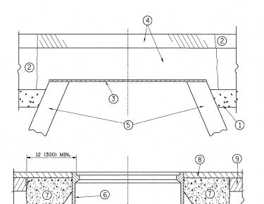
EXISTING BROKEN FRAMES AND LIDS SHALL BE REMOVED AND DISPOSED OF BY THE CONTRACTOR AND SHALL BE REPLACED AS DIRECTED BY THE ENGINEER. REPLACEMENT FRAMES AND LIDS WILL BE PAID FOR IN ACCORDANCE WITH ARTICLE 109.04 OF THE STANDARD SPECIFICATIONS UNLESS A SEPARATE PAY ITEM HAS BEEN PROVIDED.
