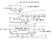
$\divideontimes$  TURN LANES IN EXCESS OF 400' (120 m) IN LENGTH MAY HAVE AN ADDITIONAL SET OF ARROW - "ONLY" INSTALLED MIDWAY BETWEEN THE OTHER TWO SETS OF ARROW - "ONLY".
