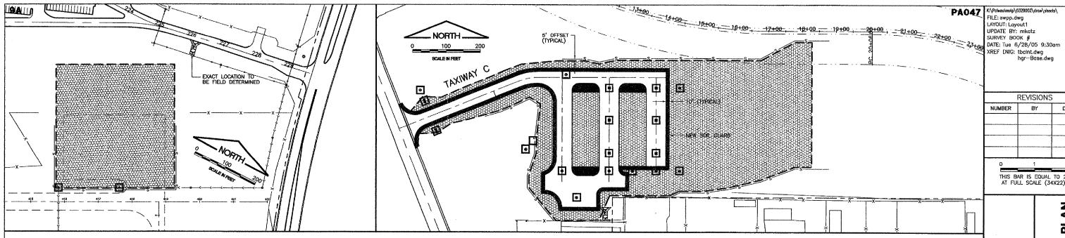
THE FOLLOWING PLAN IS ESTABLISHED AND INCORPORATED IN THE PROJECT TO DIRECT THE CONTRACTOR IN THE PLACEMENT OF TEMPORARY EROSION CONTROL SYSTEMS AND TO PROVIDE A STORM WATER POLLUTION PREVENTION PLAN FOR COMPLIANCE WITH NPDES.
