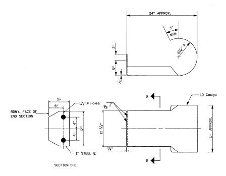
ALL OTHER STEEL SHAPES AND PLATES SHALL CONFORM TO THE REQUIREMENTS OF A.A.S.H.T.O. DESIGNATION M-183 EXCEPT POSTS AND ANGLES SHALL CONFORM TO A.A.S.H.T.O. M-223, GRADE 50.
