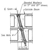
PARTIAL PLAN TRANSVERSE TIE ASSEMBLY ('D'=0°, 5° and 10°)
