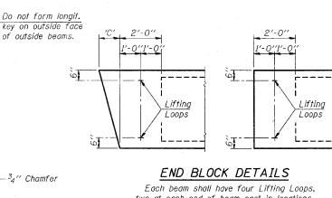
two at each end of beam cast in locations shown above. Loops shall be burned off after beams have been erected.
