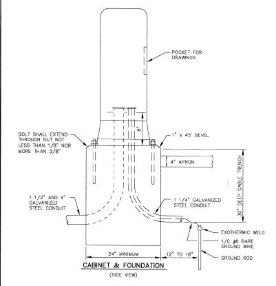
NOTE: CONCRETE FOUNDATION SHALL CONFORM TO STANDARD 878001 FOR TYPE D FOUNDATION
