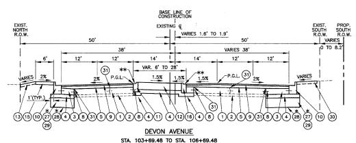
\*STA. 103+69.48 TO STA. 103+75 - 10" DEPTH (AS DIRECTED BY THE ENGINEER) STA. 103+75 TO STA. 106+69.48 - 16" DEPTH (AS DIRECTED BY THE ENGINEER)
