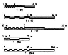
FULL SIZE PLANS HAVE BEEN PREPARED USING STANDARD ENGINEERING SCALES. REDUCED SIZED PLANS WILL NOT CONFORM TO STANDARD SCALES. IN MAKING MEASUREMENTS ON REDUCED PLANS, THE ABOVE SCALES MAY BE USED.
